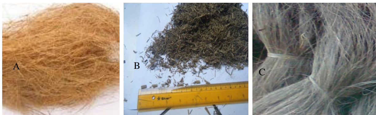
Figure 1. Raw material of three types of natural fibers (A: coconut fiber, B: rice straw, C: palm fiber)
