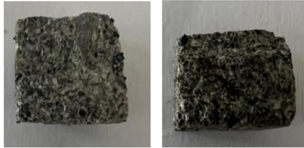
Gambar 2. Sampel Uji SEM-EDX Mapping: (a). Mortar ECC, (b.) Crumb Rubber ECC
